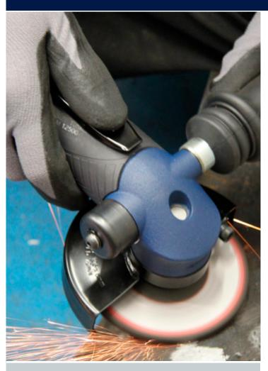
This angled grinder by Yokota is used for grinding and cutting. Very high quality level. The grinder has an integrated speed-setting regulator for maximum safety and optimal speed for best material removal. The spindle can be held by push button for easy exchange of accessories like grinding discs.
