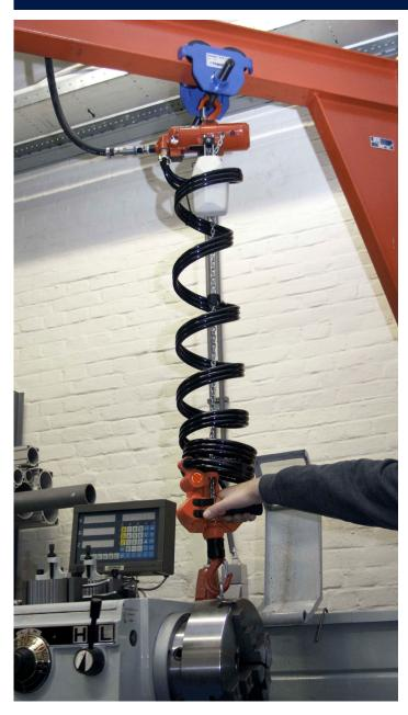
The RED ROOSTER Compact Hoists are suitable for 'Material-Handling'. The pendant control is direct on the lower hook so the operator can control and position the load easy and direct. The perfect solution for horizontal movements is the combination with a push trolley.
