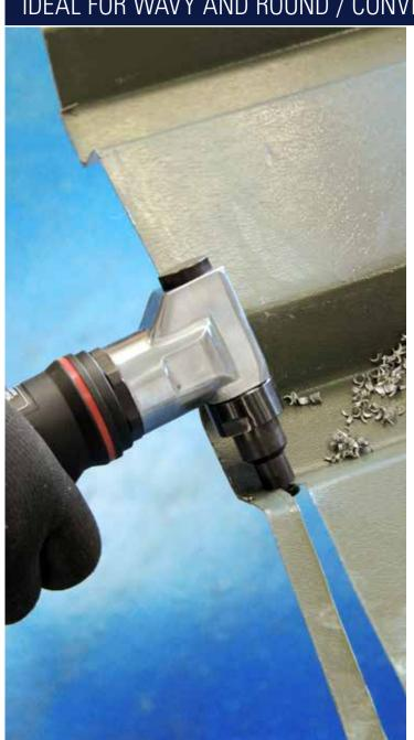
The Red Rooster RR-8116 nibblers are quick, easy to maneuver to cut circles, curves and corners in sheet metal and bodywork. Also ideal for wavy and round / convex sheet metal work. The cut sheet metal is not deformed. The head can be adjusted in four steps of ninety degrees to fit perfectly to the workpiece.
