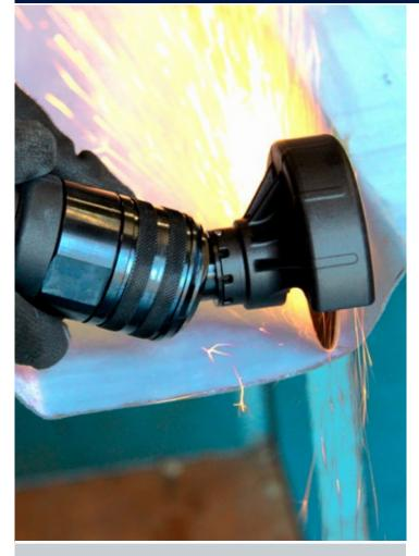
This RED ROOSTER power cutter is used with 75 mm cutting discs. By this flexible tilting head, hard-to-reach places are more accessible, this maximizes the ergonomic properties and allows you to use a high precision grinding. This tool has a very powerful air motor of 600 Watt. Very suitable for precise cutting of, for example, sheet steel, body parts and exhaust pipes.
