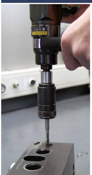
The RED ROOSTER universal tapping machine RRI-T330M12 has been developed for manual thread tapping. The direction of rotation and speed are easily adjusted with the rocker switch. It is an ergonomically developed tool that fits well in the hand. Exhaust through grip, sound muffled. Thanks to the quick-change holder, different sizes of tap holders can be changed quickly and easily.
